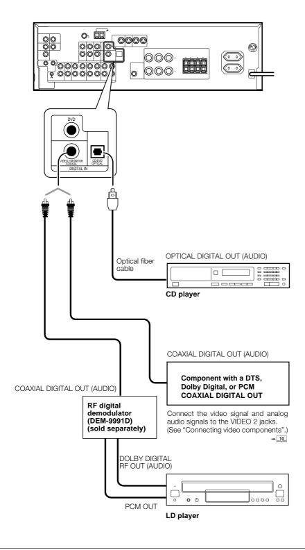
To connect an LD player with a DIGITAL RF OUT, connect the LD player to the KENWOOD RF digital demodulator (DEM-9991D). Next, connect the DIGITAL OUT jacks of the demodulator to the DIGITAL IN jacks of the receiver. Connect the video signal and analog audio signals to the VIDEO2/MONITOR jacks. (See "Connecting video components".)
